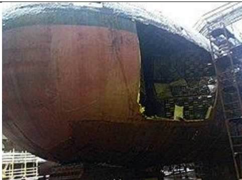
For repairs, workers cut a large hole in the lightweight hull Photo: forums.airbase.ru
