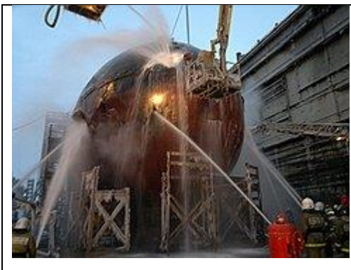
Mid-afternoon December 30: Firefighters continue to flood the fire through emergency and emergency holes in the light hull
